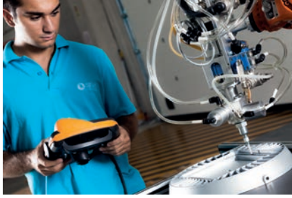
► Armatür Contalama Robotu Product Sealing Robot
