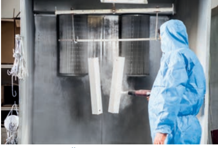
► Toz Boyama Ünitesi Electrostatic Powder Coating Unit
